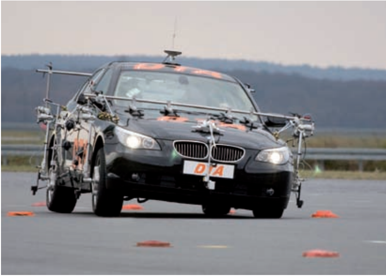
Figure 4: Vehicle maneuvers: VDA obstacle avoidance test
