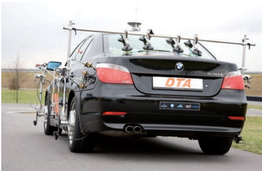
Figure 1: Exterior view of the measuring instrumentation installed on the vehicle
